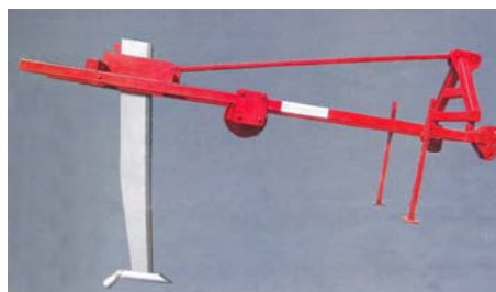
Figure 4. Drainage plough DP-4
